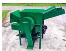
Pictorial view of the developed buckwheat thresher
